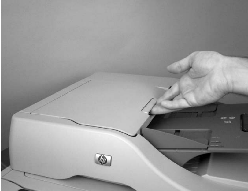
Figure 6-5 Remove the ADF input tray (1 of 3)
