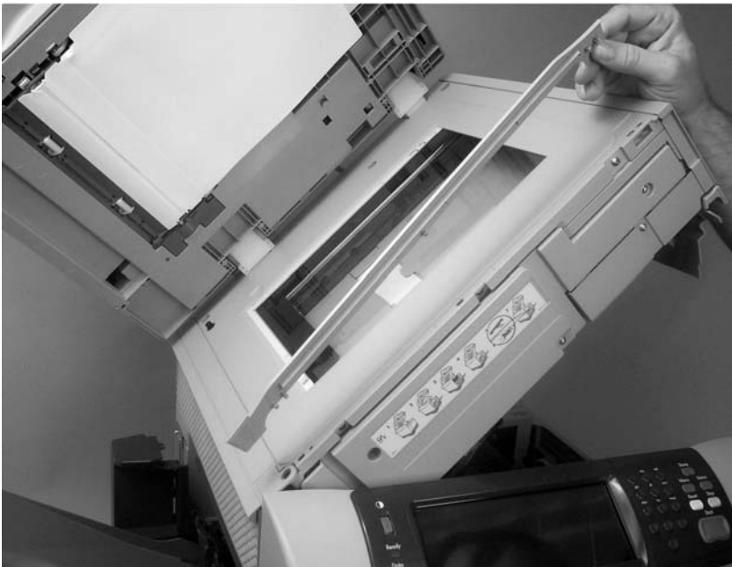
Figure 6-39 Remove the top-cover flatbed flange (2 of 2)
