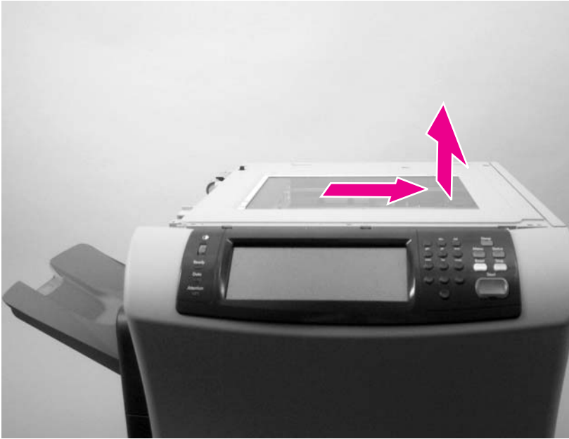
Figure 6-179 Remove the scanner assembly (8 of 8)
