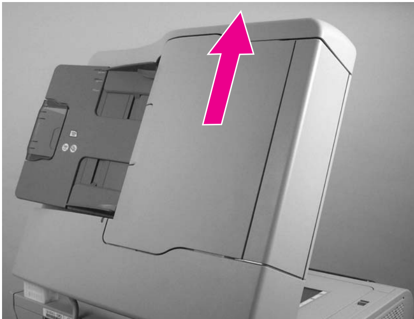
Figure 6-171 Remove the ADF assembly (3 of 3)
