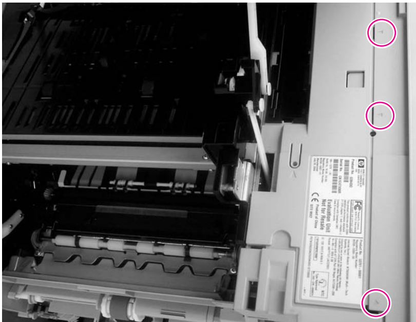
Figure 6-48 Remove the back cover (2 of 3)
