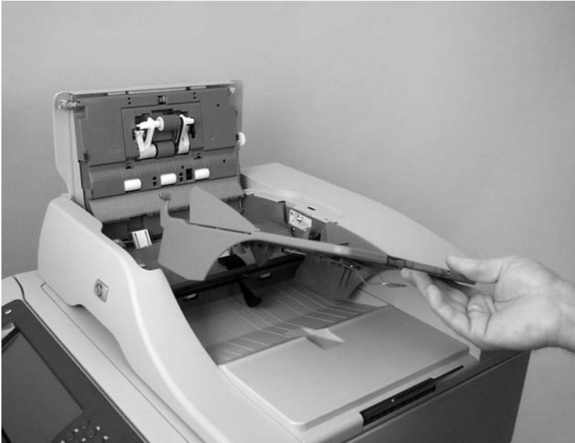
Figure 6-7 Remove the ADF input tray (3 of 3)
