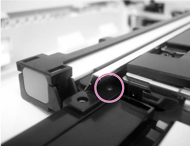
Figure 6-193 Remove the optical unit (7 of 7)
