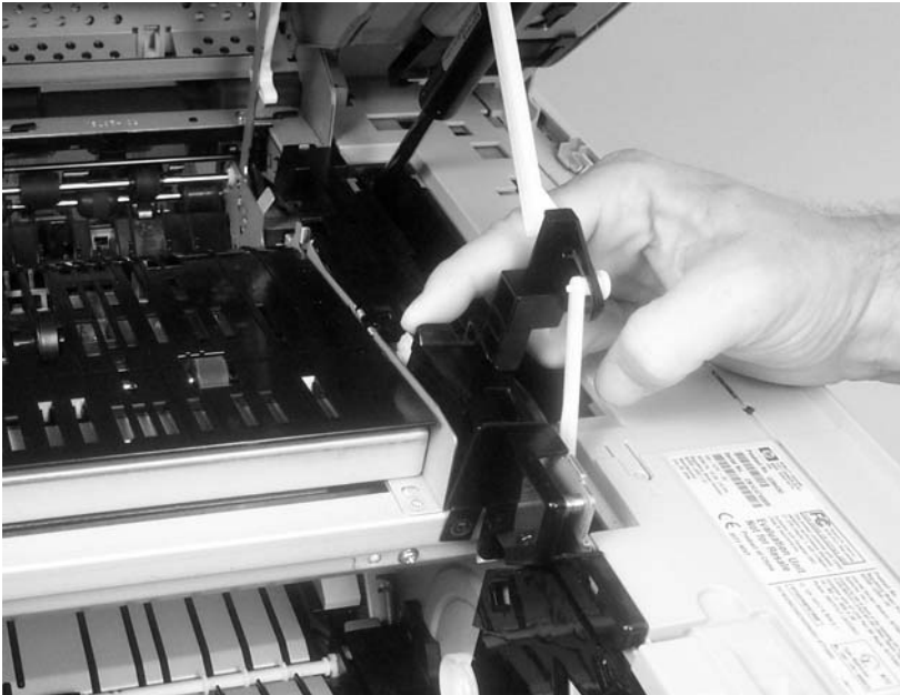
Figure 6-53 Remove the reversing assembly (2 of 8)
