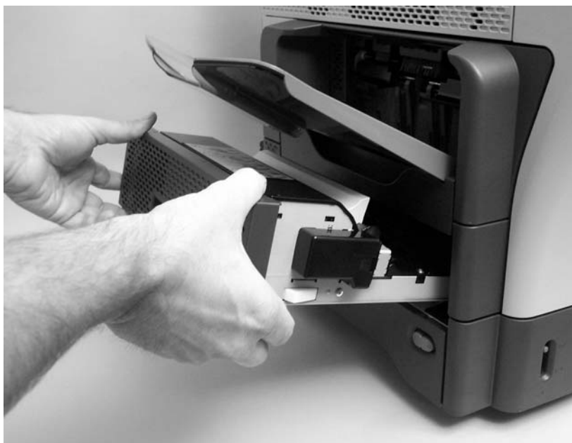
Figure 6-19 Remove the duplex-printing unit (2 of 2)
