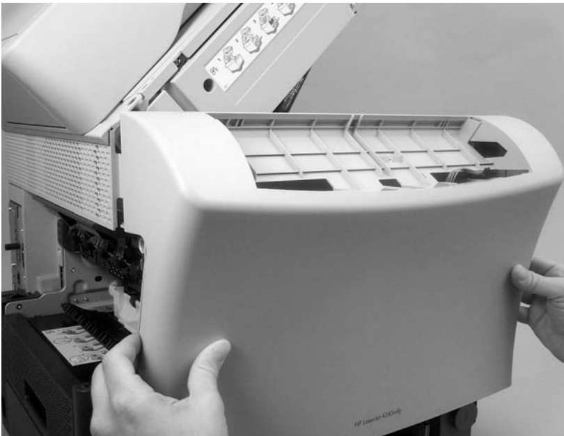
Figure 6-46 Remove the front cover (7 of 7)
