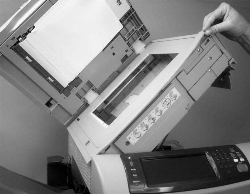
Figure 6-38 Remove the top-cover flatbed flange (1 of 2)
