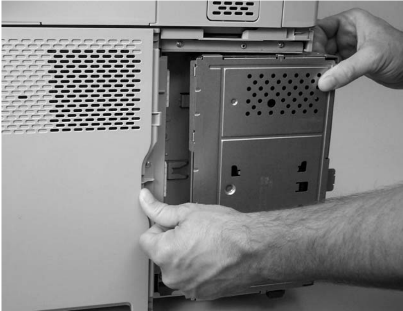
Figure 6-32 Remove the formatter cover and formatter (3 of 3)
