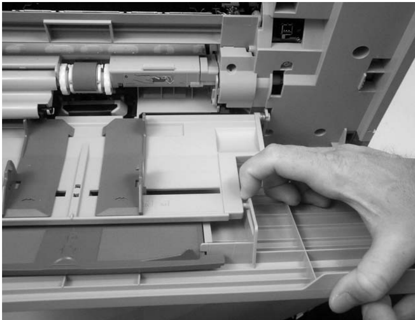
Figure 6-76 Remove the tray 1 assembly (1 of 5)
