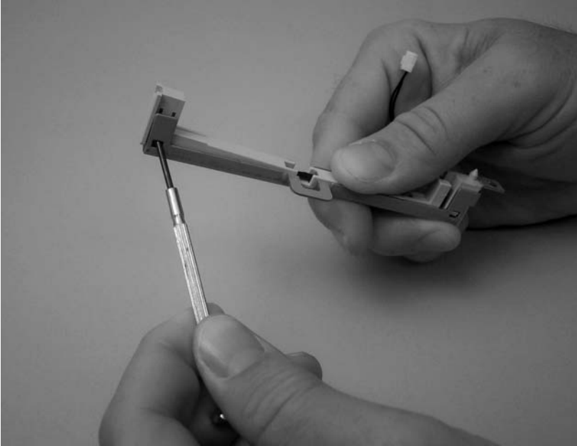
Figure 6-71 Remove the thermistor (3 of 4)
