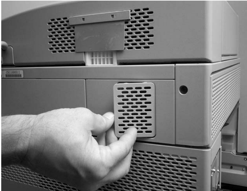
Figure 6-25 Remove the scanner filter (1 of 2)
