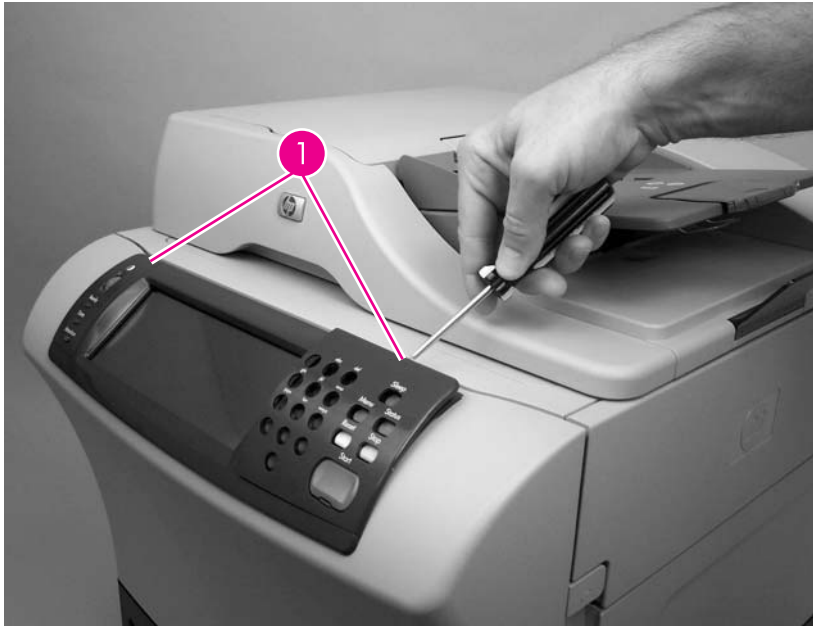
Figure 6-1 Remove the control-panel overlays
