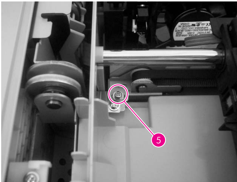
Figure 6-189 Remove the optical unit (3 of 7)
