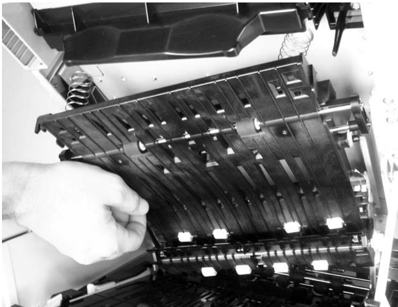
Figure 6-51 Remove the reversing-separation-guide assembly (2 of 2)
