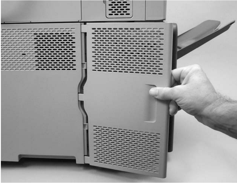
Figure 6-30 Remove the formatter cover and formatter (1 of 3)
