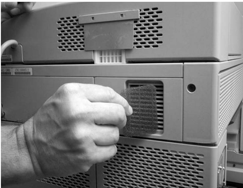
Figure 6-26 Remove the scanner filter (2 of 2)
