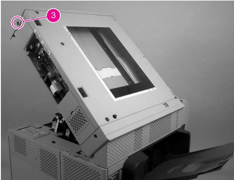
Figure 6-174 Remove the scanner assembly (3 of 8)
