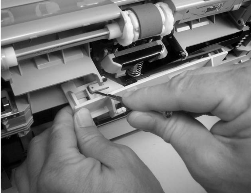
Figure 6-82 Remove the front-cover support (1 of 2)
