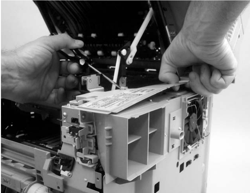
Figure 6-91 Remove the tray 1 feed-assembly (8 of 13)
