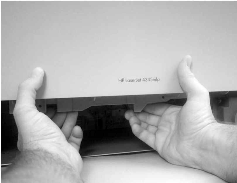
Figure 6-45 Remove the front cover (6 of 7)
