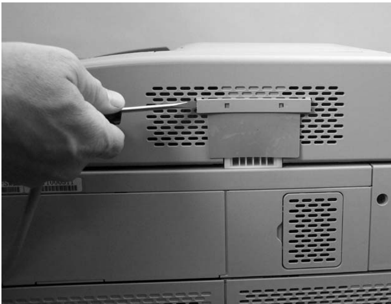
Figure 6-28 Remove the ADF-hinge flap (2 of 3)
