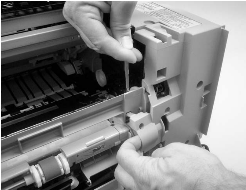
Figure 6-88 Remove the tray 1 feed-assembly (5 of 13)
