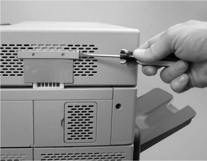
Figure 6-27 Remove the ADF-hinge flap (1 of 3)
