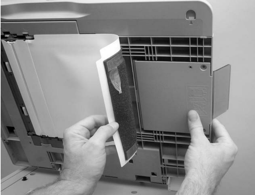
Figure 6-203 Remove the ADF output-bin extension (2 of 2)
