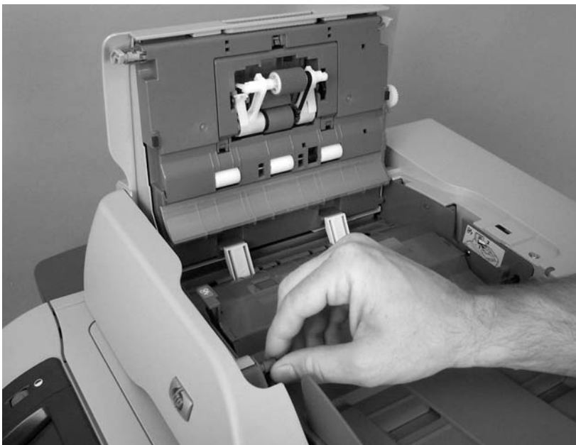
Figure 6-6 Remove the ADF input tray (2 of 3)
