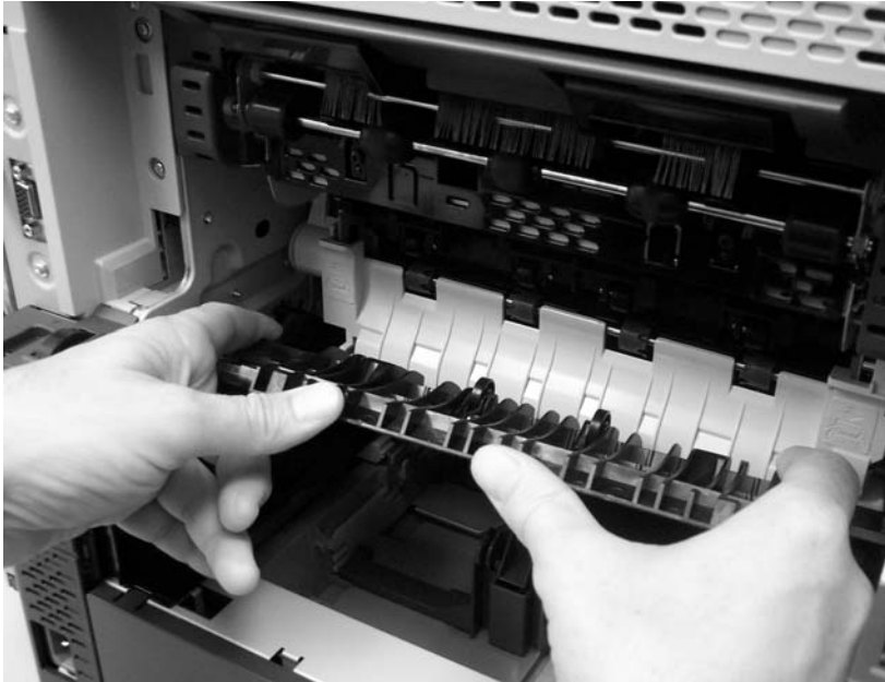
Figure 6-20 Remove the fuser-entrance guide
