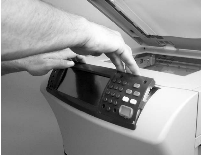
Figure 6-2 Remove the control panel (1 of 2)
