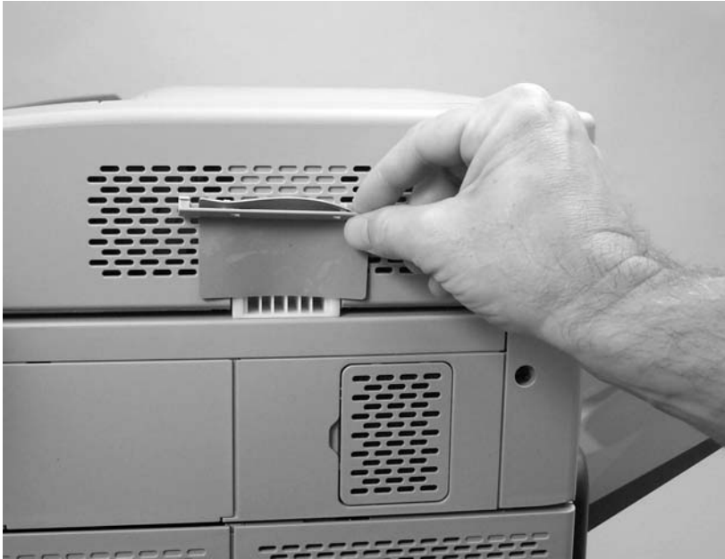
Figure 6-29 Remove the ADF-hinge flap (3 of 3)
