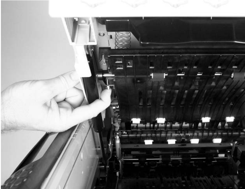
Figure 6-50 Remove the reversing-separation-guide assembly (1 of 2)
