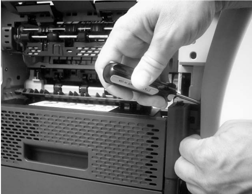
Figure 6-43 Remove the front cover (4 of 7)
