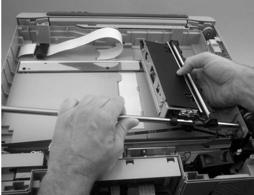
Figure 6-191 Remove the optical unit (5 of 7)
