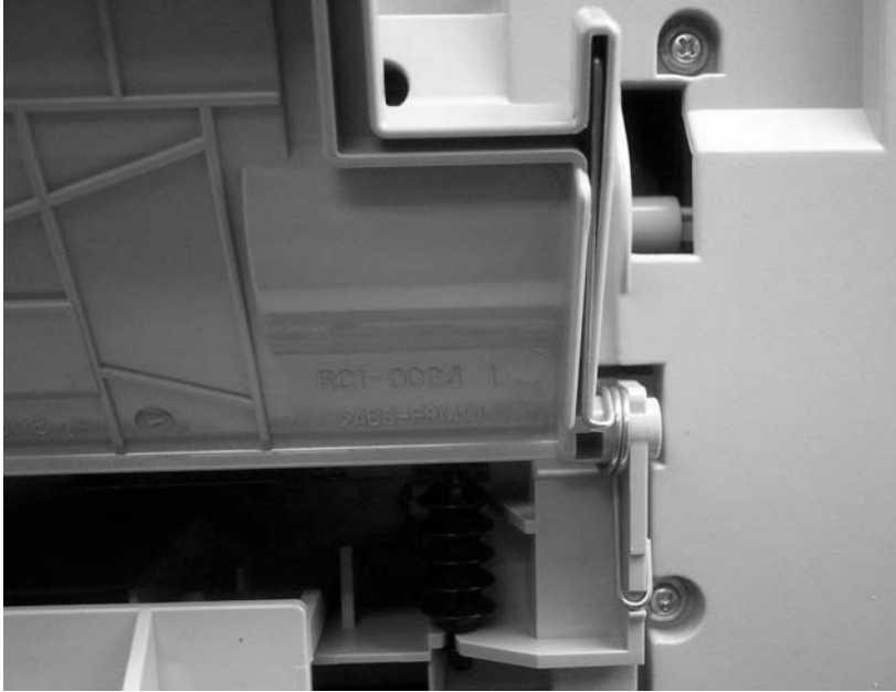
Figure 6-80 Correct tray 1 rear-hinge-spring placement
