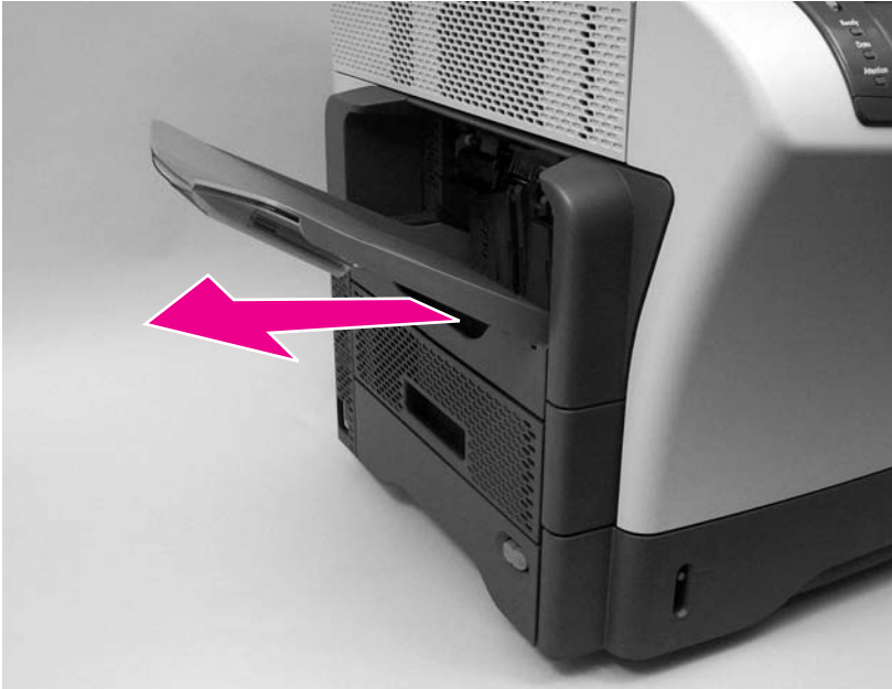
Figure 6-16 Remove the output-bin assembly (1 of 2)
