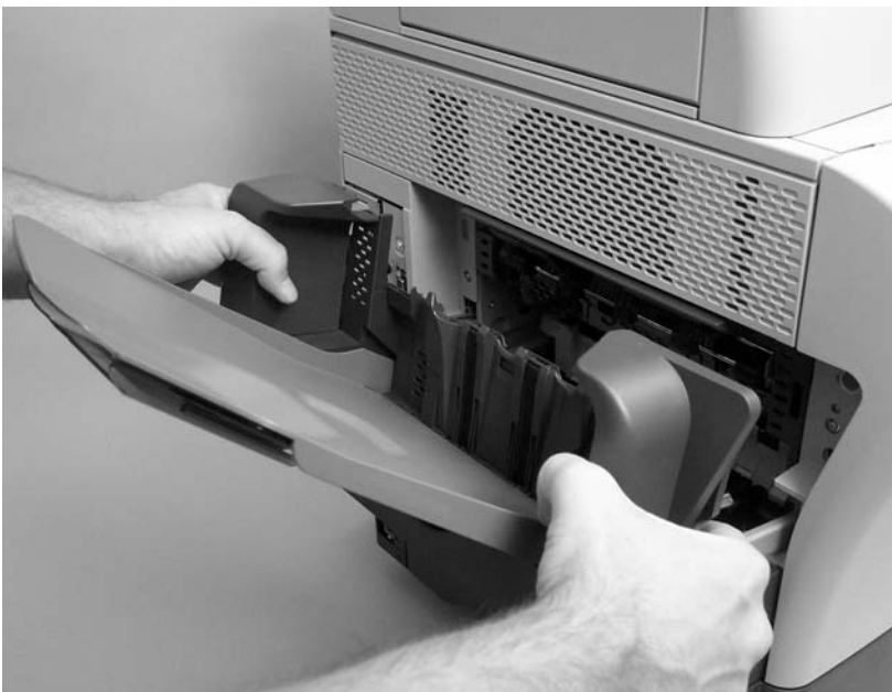
Figure 6-17 Remove the output-bin assembly (2 of 2)
