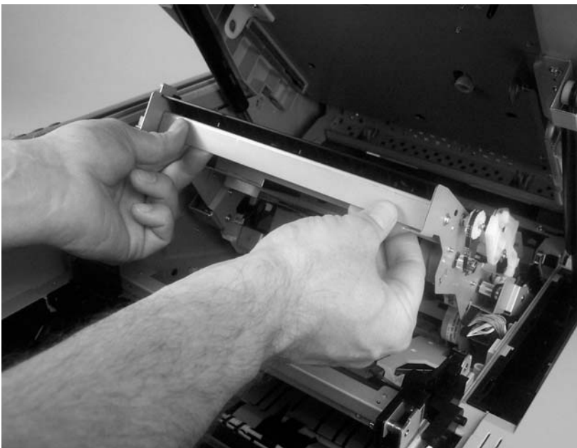
Figure 6-59 Remove the reversing assembly (8 of 8)
